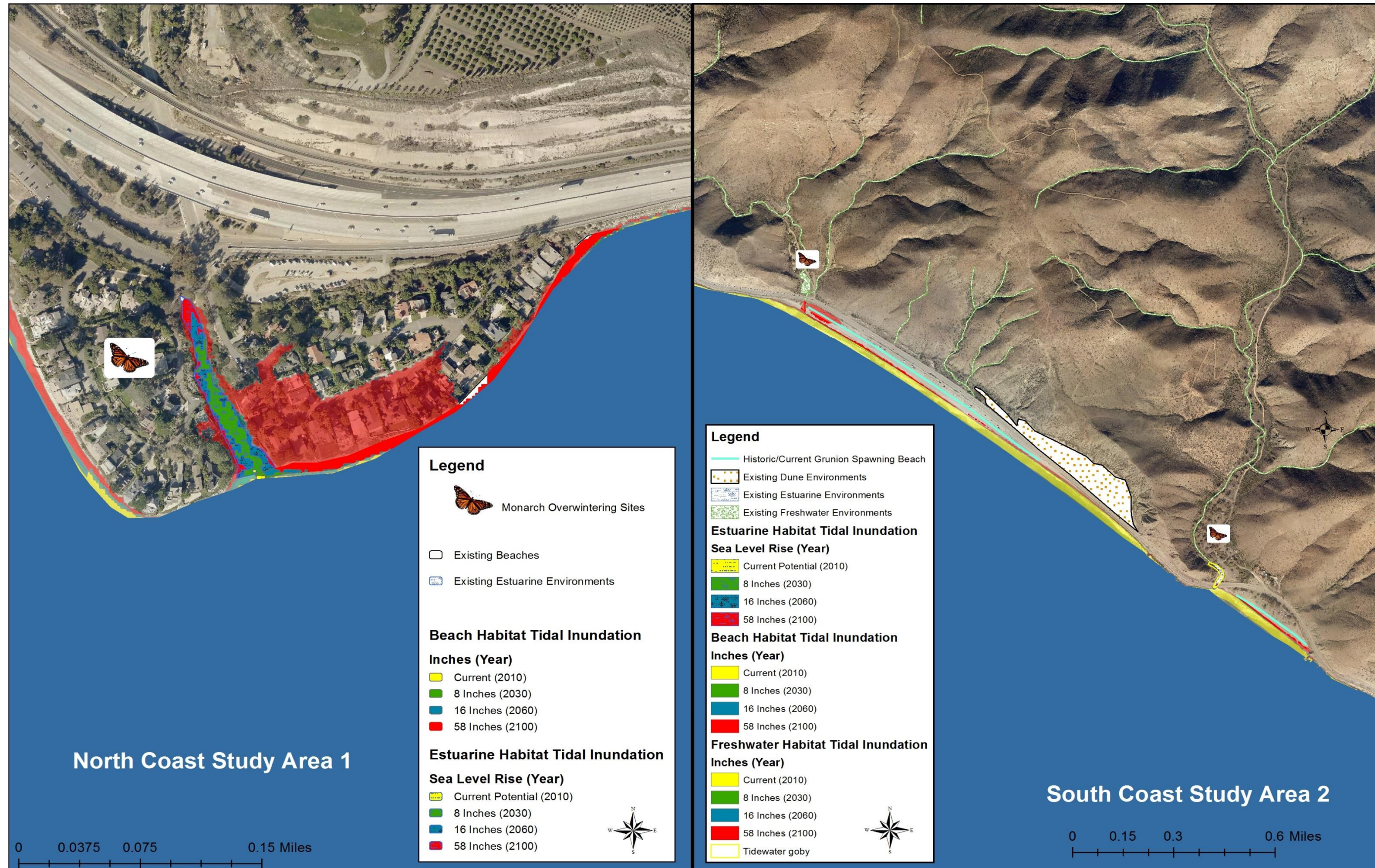
Figure D-15. North Coast Projected Tidal Inundation Due to Sea Level Rise (Study Areas 1 and 2)
