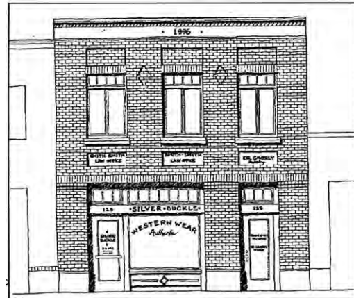
Window Proportions – at street level, openings should be 50% to 60% of the face, with 30% to 50% at the second floor.
