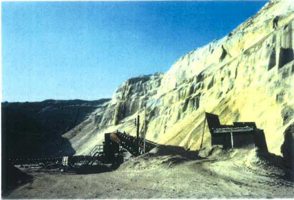
Photo No. 4 View of active mining area. Material is pushed down the slope and loaded into hopper for transport by conveyor belt.
