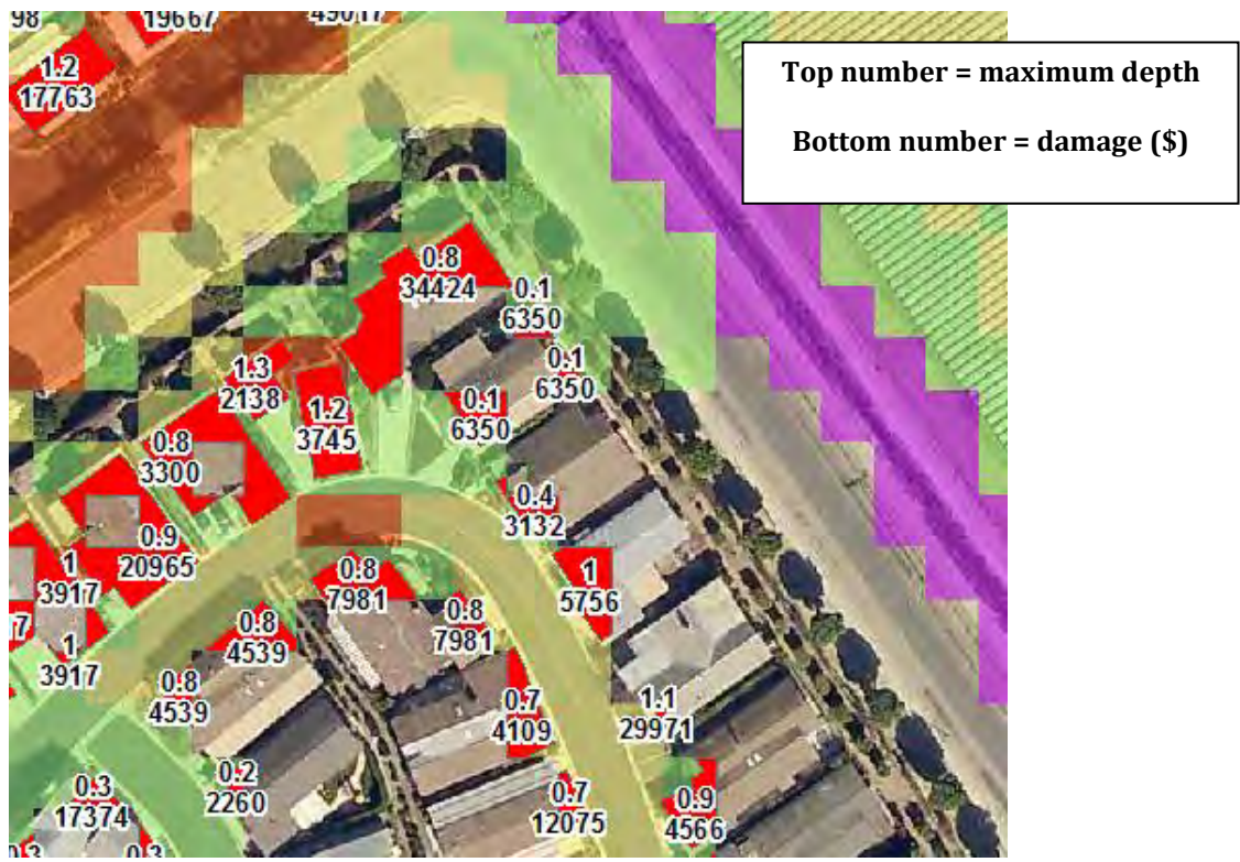
Figure 23 100-Year Event Damage Overlay Example
