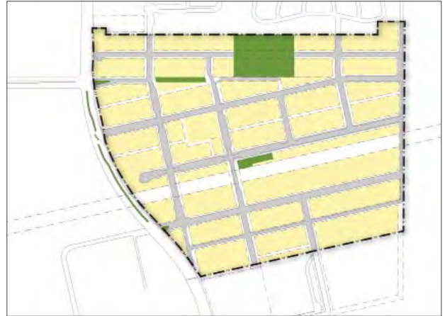
Phase 1. Parks are introduced on the County-owned stormdrain pipe right-of-way and adjacent to the old Saticoy Depot. The area of the two new parks is 0.8 acres.
