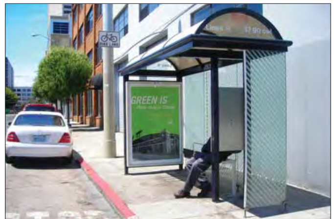
A simple bus stop with a bench, shelter, lighting, and signage
