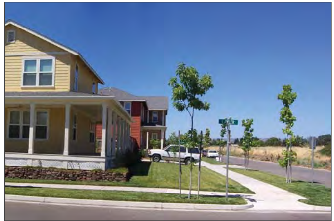
Example of a residential street as the edge of town. Sidewalks and street trees are introduced on one side of the street.
