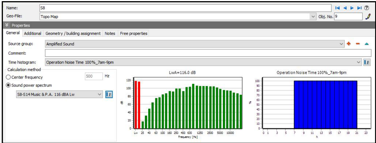
Figure 6. Amplified Sound Source Data for S8, S9, S10, S11, S12, S13 and S14
